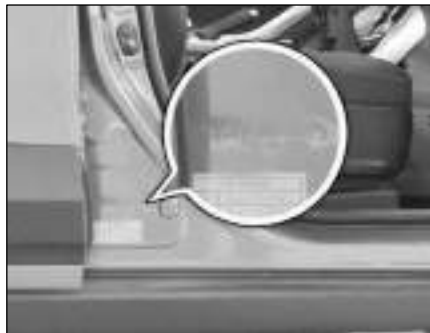
Chassis No. punching near driver seat
