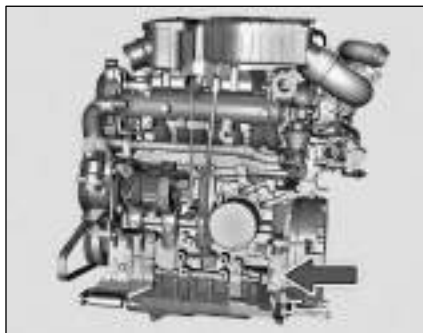
Engine No. Plate - Diesel
