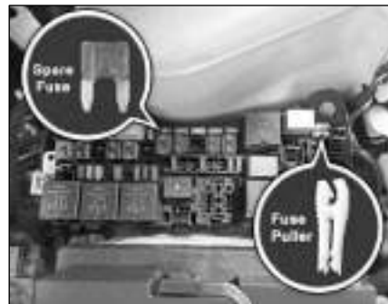
Engine compartment fuse box
