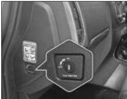
PAB deactivation switch
